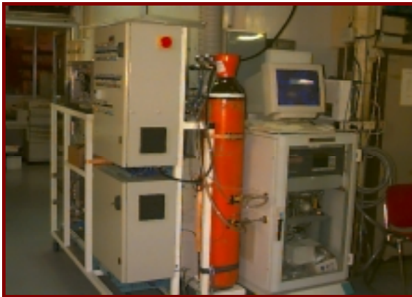
Figure 3 – Bench for the measurement of refrigerant leak flow rates.
